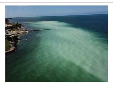
Figure 1. Sediment pollution due to coastal works dredging for Heritage Holdings Ltd, 2017.
