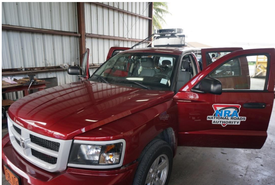
Figure 5 Photograph of the NRA provided vehicle mounted with SEMIC survey equipment
