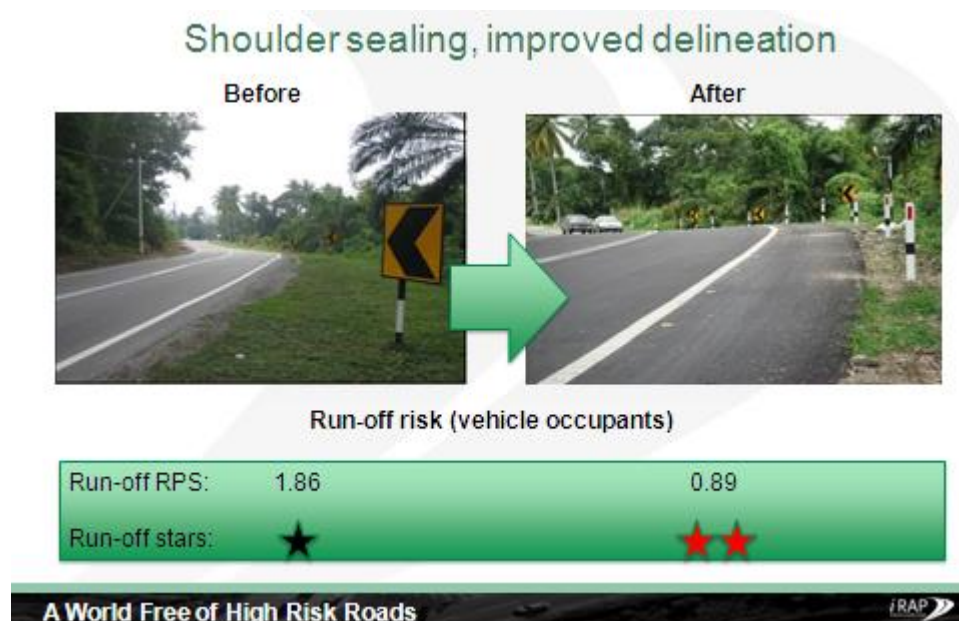
Figure 20 Example of a Safety Improvement Project Showing the Star Rating Before and After Improvement
