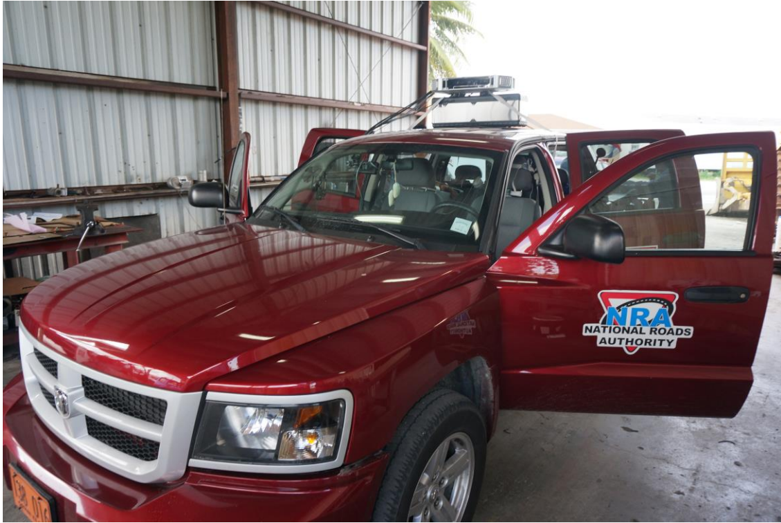
Figure 11 Photograph of the NRA provided vehicle mounted with SEMIC survey equipment
