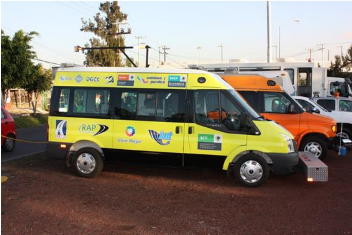
Figure 2 - iRAP accredited survey vehicle used in Mexico
