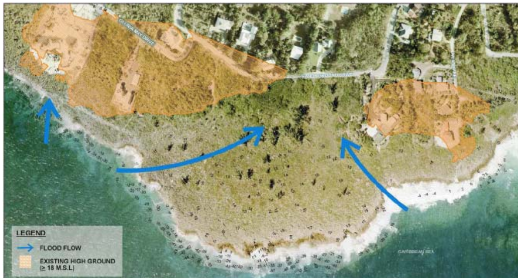
Seawater infiltrates ironshore at Savannah Acres then flows downhill into parts of the Savannah/Newlands community.
