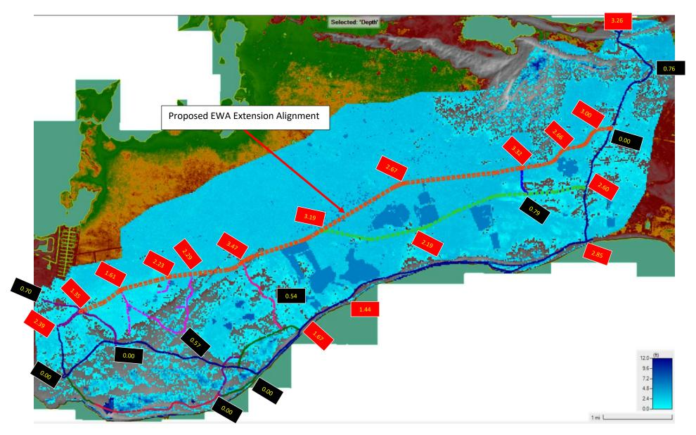
Figure 14 Maximum flood depth, in feet, for 24 hours event with a 100 years return period (Black highlighted less than 1ft, Red highlighted more than 1ft)
