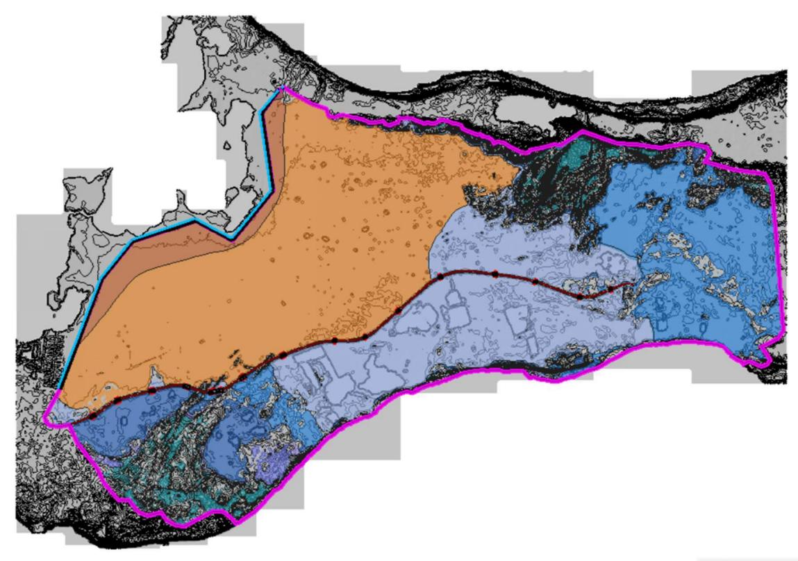
100-Year Storm Maximum Water Surface Elevations With Model Terrain
