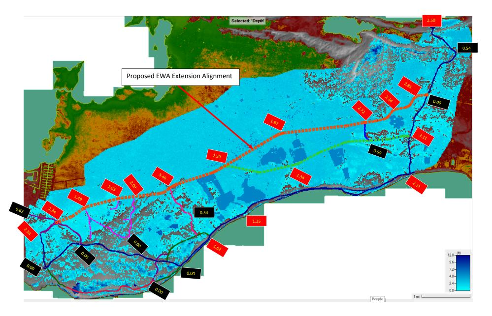
Figure 13 Maximum flood, in feet, depth for 24 hours event with a 50 years return period (Black highlighted less than 1ft, Red highlighted more than 1ft)
