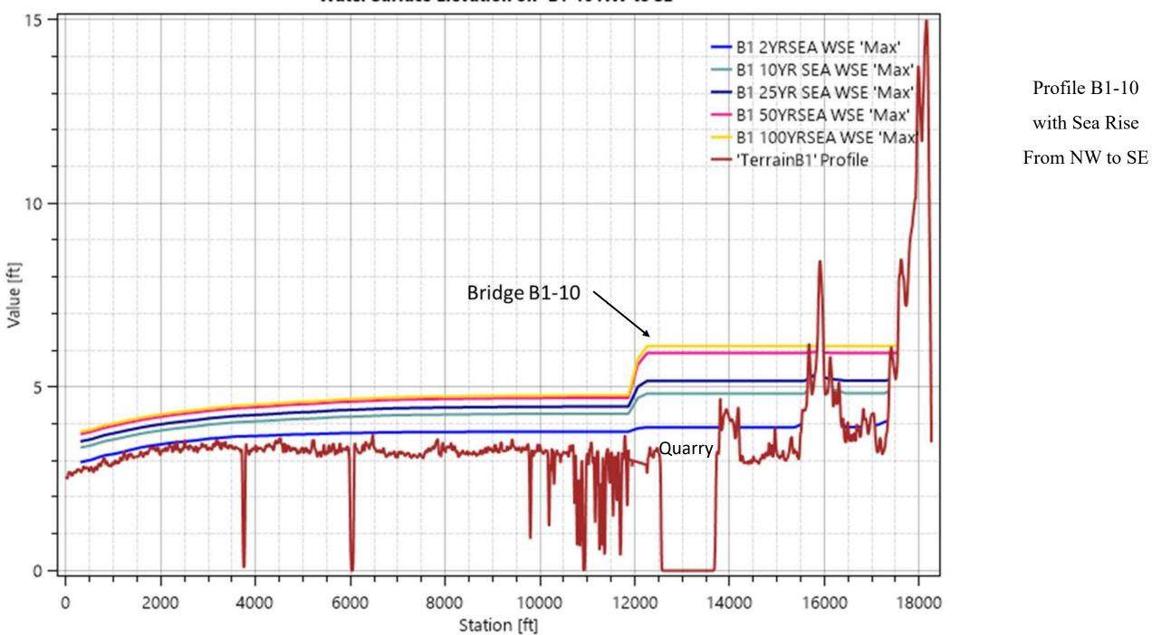
Water Surface Elevation on 'B1-10 NW to SE'
