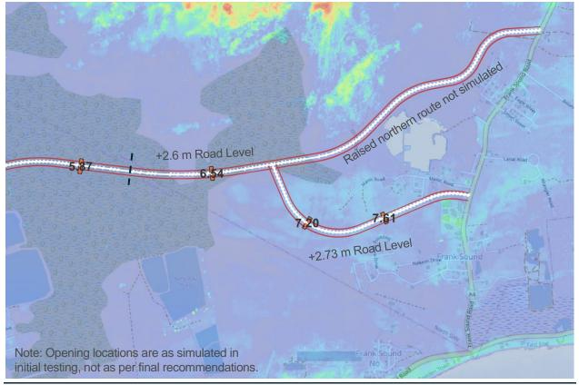
Figure 6.3: Elevations and Simulated Openings for Eastern Section
