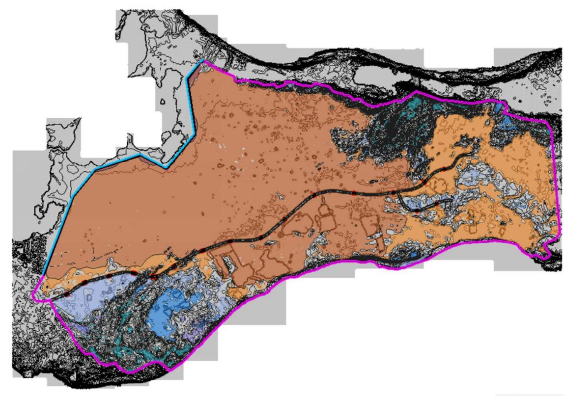
2-Year Storm Maximum Water Surface Elevation and Model Terrain
