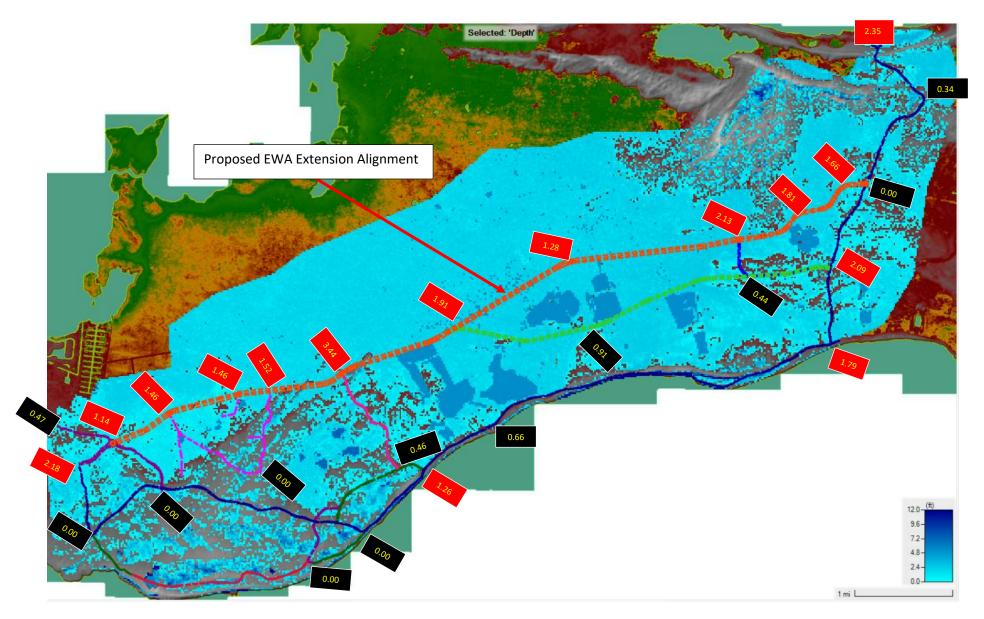
Figure 12 Maximum flood depth, in feet, for 24 hours event with a 25 years return period (Black highlighted less than 1ft, Red highlighted more than 1ft)
