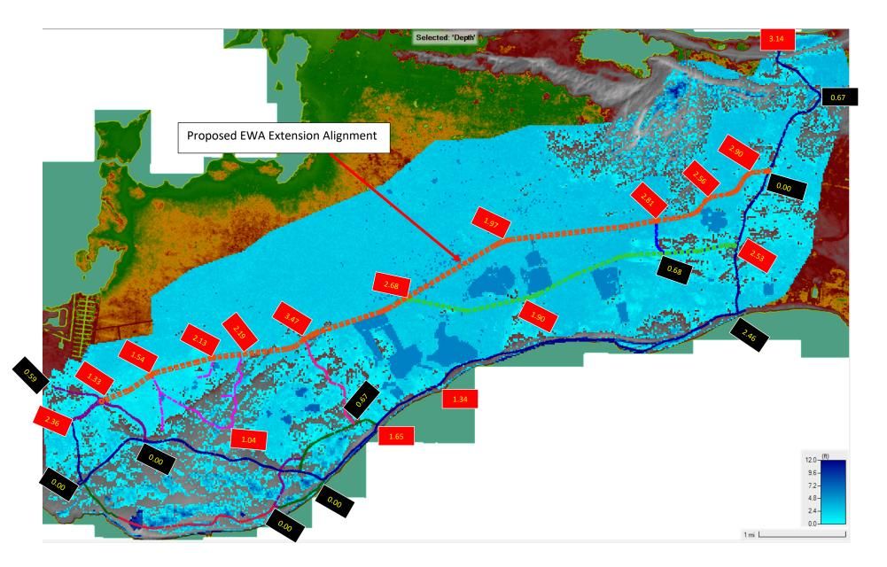
Figure 15 Maximum flood depth, in feet, for 24 hours event with Hurricane Ivan of 2004 (Black highlighted less than 1ft, Red highlighted more than 1ft)
