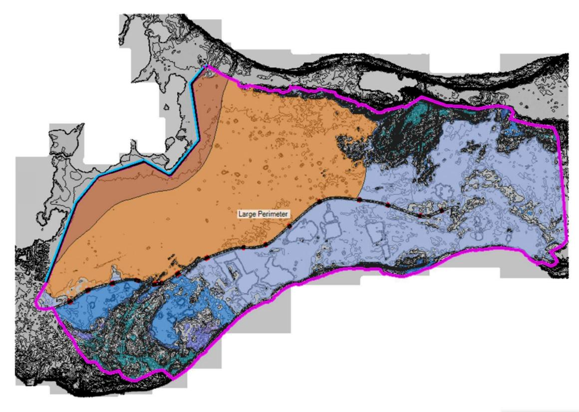
25-Year Storm With Sea Rise Maximum Water Surface Elevations With Model Terrain
