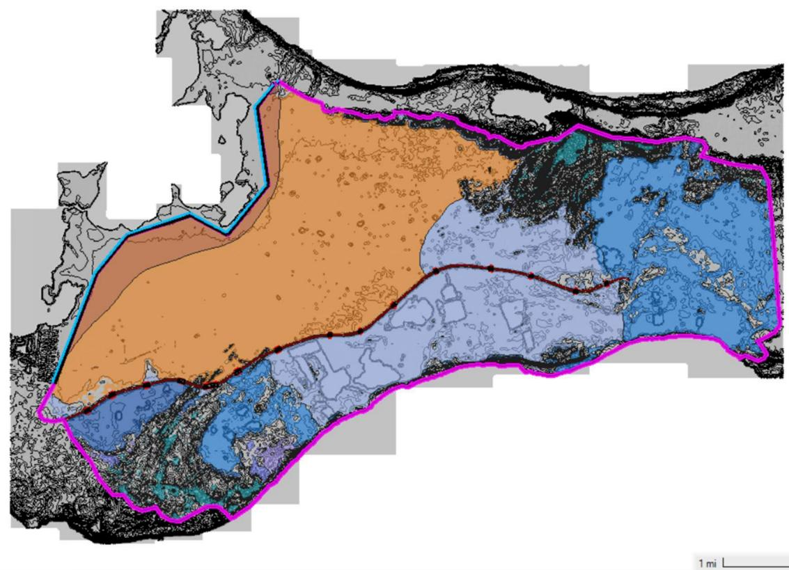
100-Year Storm With Sea Rise Maximum Water Surface Elevations With Model Terrain
