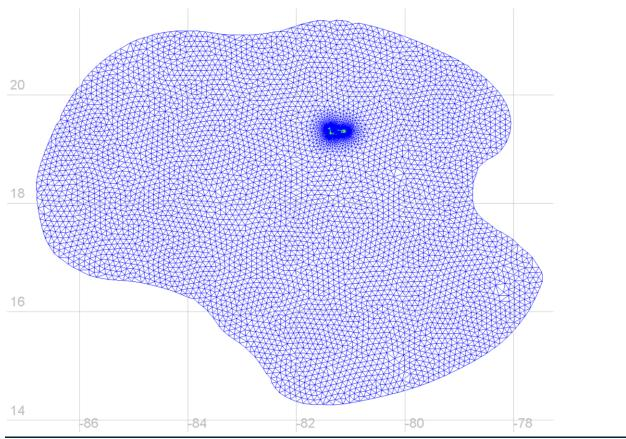
Figure 2.2: Model Domain for Telemac Simulations of Grand Cayman
