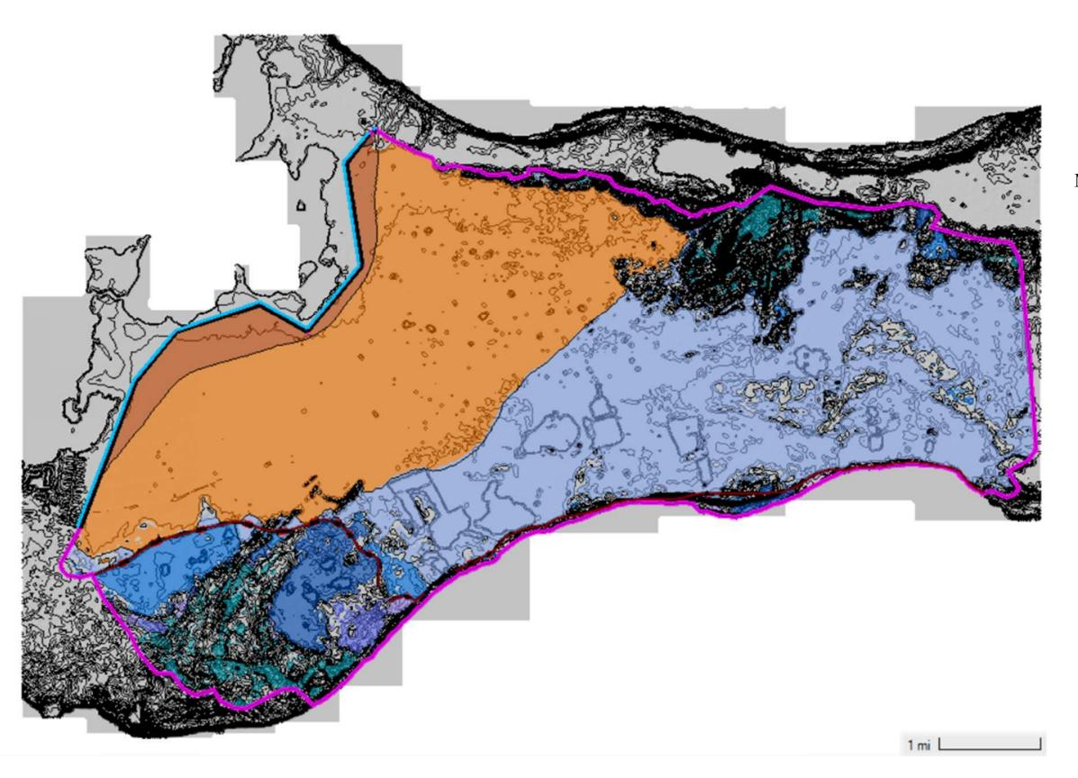
50-Year Storm Maximum Water Surface Elevations With Model Terrain
