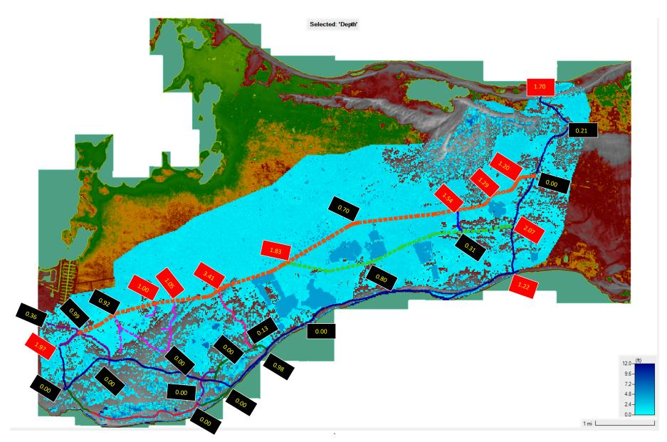
Figure 11 Maximum flood depth, in feet, for 24 hours event with a 10 years return period (Black highlighted less than 1ft, Red highlighted more than 1ft)
