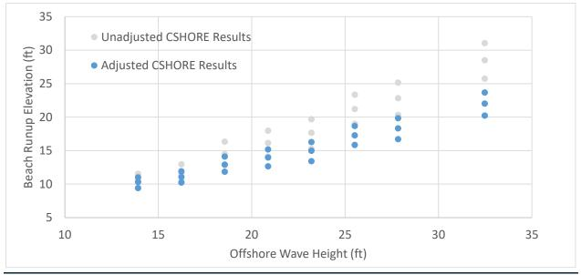
Figure 4.5: Unadjusted and Adjusted CSHORE Runup Estimates
