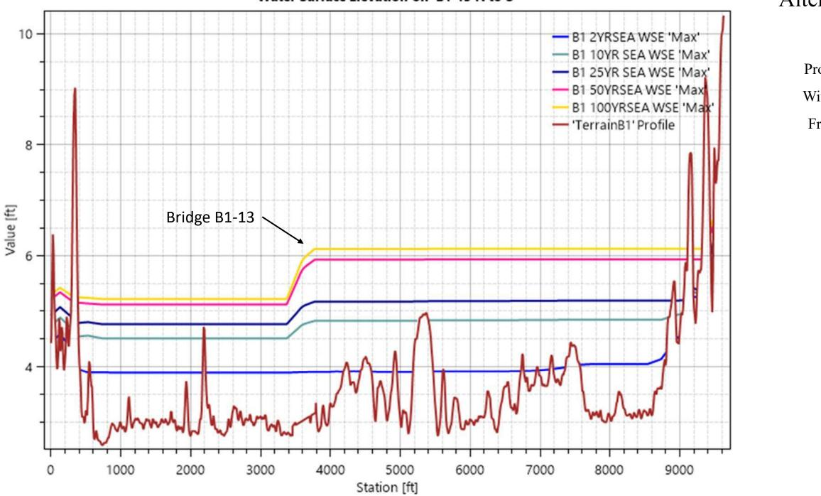
Water Surface Elevation on 'B1-13 N to S'
