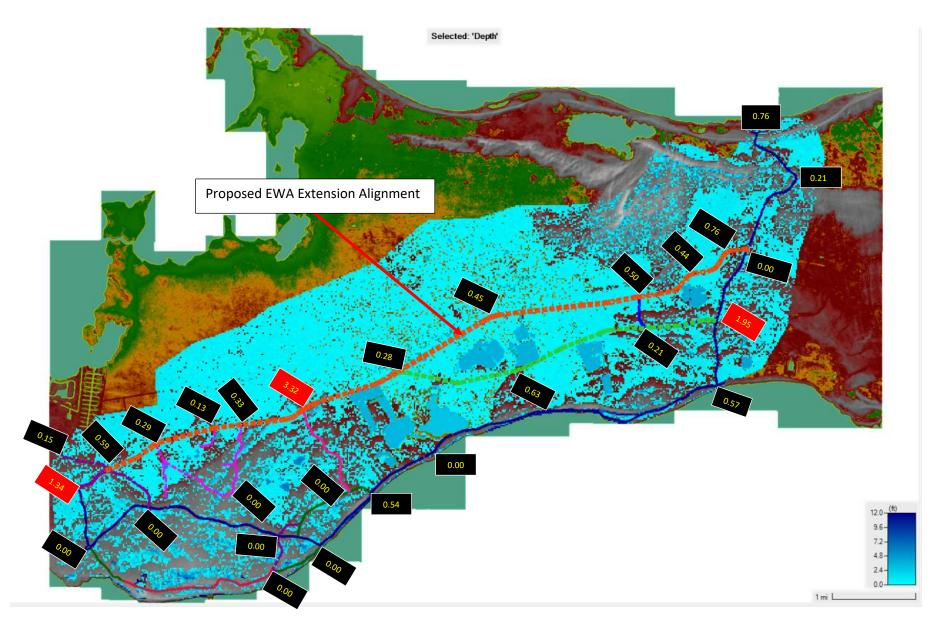
Figure 10 Maximum flood depth, in feet, for 24 hours event with a 2 years return period (Black highlighted less than 1ft, Red highlighted more than 1ft)
