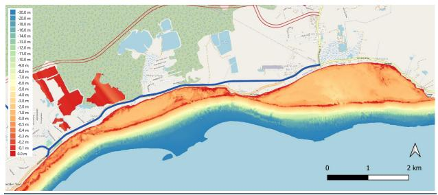
Figure 4.1: Nearshore Bathymetric Conditions Along B4 Alignment
