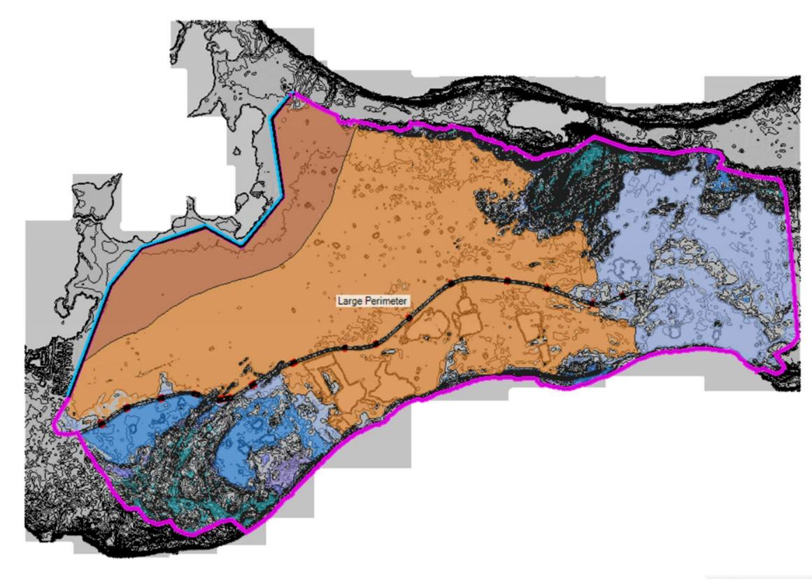
10-Year Storm Maximum Water Surface Elevations With Model Terrain
