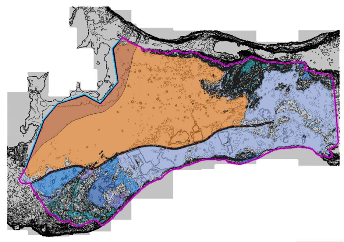
25-Year Storm Maximum Water Surface Elevations With Model Terrain
