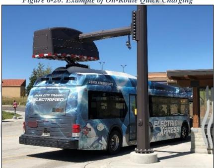
Figure 6-20: Example of On-Route Quick Charging
