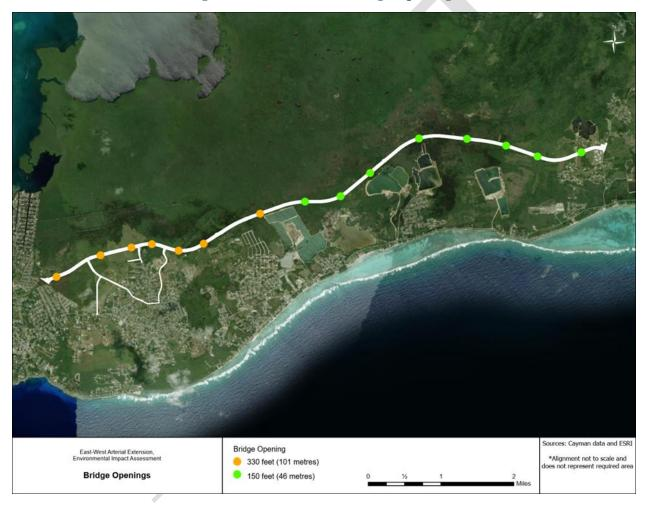
Figure 12-16: Modelled Bridge Openings
