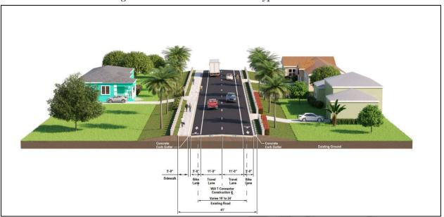
Figure 8-10: Will T Connector Typical Section
