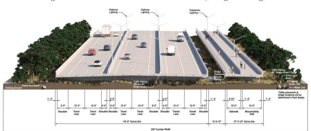
Figure 7-14: 2074 Section 2 and 3 Cross-Section, Bridge Crossings
