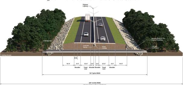
Figure 7-12: 2026 Section 2 and 3 Cross-Section
