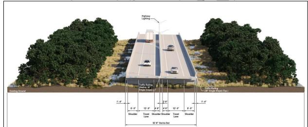
Figure 6-6: Bridge Typical Sections for Proposed Project
